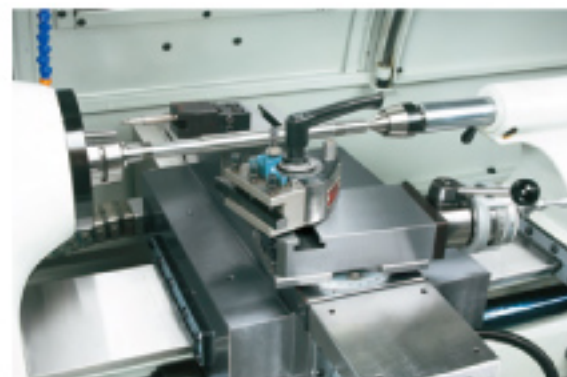
Lathe center in tailstock single tool on quick change tool holder on compound slide.
