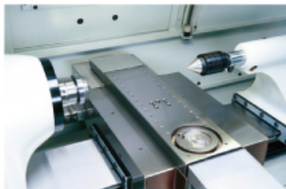
Bare cross slide with precision locator holes for custom applications.
