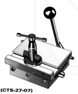
The straight and taper turning slide can be used on the front or rear of the double tool cross slide. It is for straight or angular turning, back facing, undercutting or for turning long slender parts that cannot be readily formed by a full width tool. Two of the attachments may be mounted on the double tool cross slide for turning or boring two different angles at one setting of the work, such as valve seats or bevel gears.
